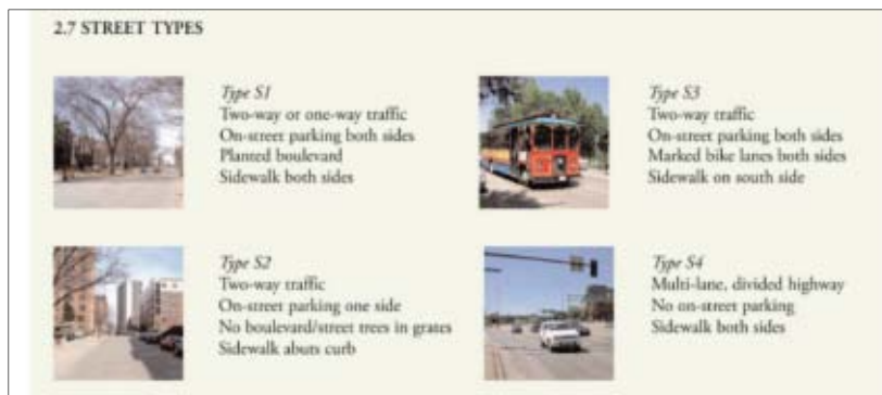
Figure above is cropped from the Loring Hill Design Guidelines (2006). There are four desired Street Types S1-S4 specified in the Loring Hill Design Guidelines .
